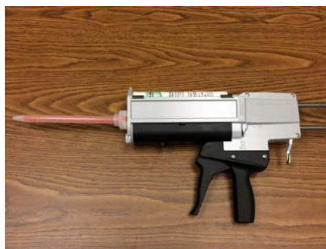
14. The assembled dispensing gun is now ready for use. Note: the adhesive inside the mixing tip may cure if the tip is left on the cartridge for a prolonged duration without additional use. In this case, keep the mixing tip on the cartridge. When you are ready to dispense the adhesive again, replace the mixing tip. Dispense and discard 1 – 2 inches of the adhesive prior to use.
