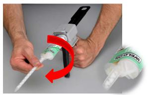
Insert the mixing tip to the cartridge and turn clockwise ¼ turn to lock the mixing tip onto the cartridge.
