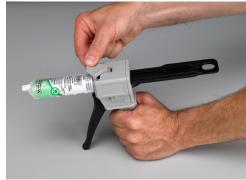
6. Press the gray lever down to lock the cartridge onto the dispensing gun.
