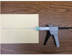
10. Squeeze the black lever and dispense approximately 1 to 2 inches to ensure both components of the adhesive are completely mixed before use.
