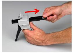
2. Hold the metal lever and pull the black plunger forward.
