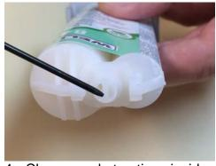
4. Clear any obstructions inside the nozzle openings with a probe. Place the white cap back on the cartridge and turn clockwise ½ turn.
