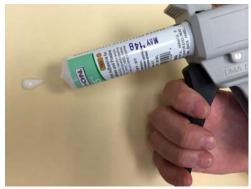
8. Squeeze the black lever and dispense a small amount of adhesive making sure that both components flow freely from the cartridge nozzle.
