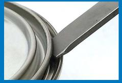
Flat-edge handle is used to open paint-style solvent cement cans.
