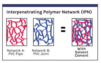
When solvent cement is applied it loosens the interpenetrating polymer network (IPN) molecules so they can be entangled to create a bond stronger than the pipe.
