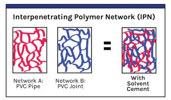
When solvent cement is applied it loosens the interpenetrating polymer network (IPN) molecules so they can be entangled to create a bond stronger than the pipe.
